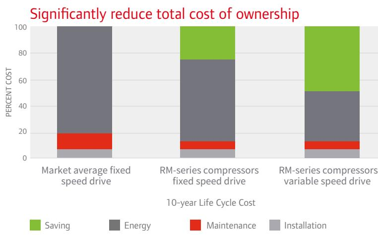
Rotary comparison at 79% average volume capacity; 4000 hours per year; 0.05\$/kWh
